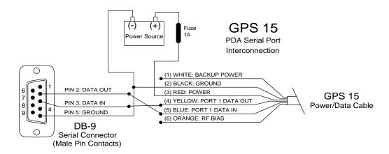
**Figure 2. PDA Serial Port Interconnection**
